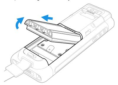
8. Loosen the screws securing the card access door closed. Use the tab to lift the edge of the door.
