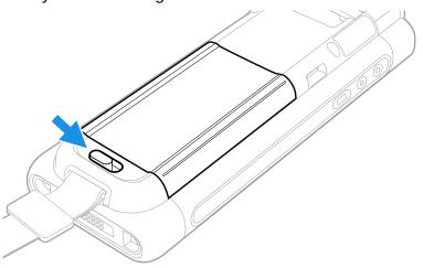
6. Lift up on the edge of the battery and remove it from the computer
