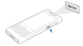
4. Release the Scan button when the computer beeps, and the Scan Status LED briefly turns on. The bar code information is entered into the application in use.
