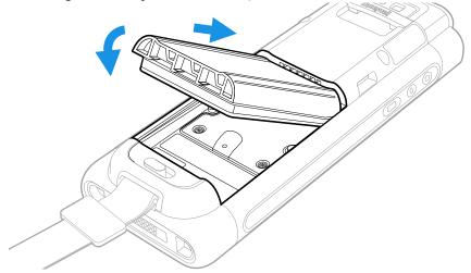
8. Press down on the edge of the battery to engage the lock.
