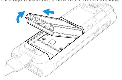
7. Insert the charged battery into the computer.
