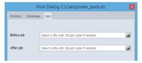
The  ${\tt Job}$  tab, allow to send files with JScript code, to run on printer before or after printing a label.
